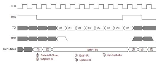
Figure 5-9 Data Register Access Timing
