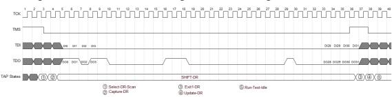
Figure 5-12 Read ID Code Data Register Access Timing
