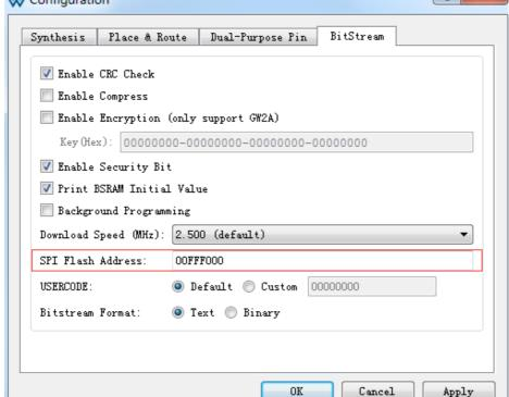
Select the external Flash mode in Programmer, set the start address of BitStream. This address should be the same as the start address set in
