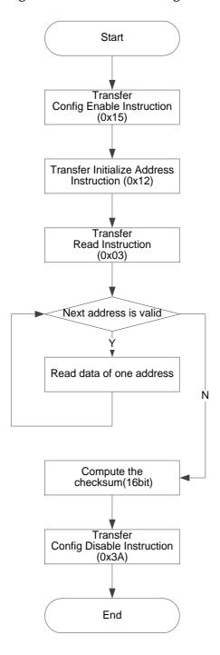
Figure 5-14 Process of reading SRAM
