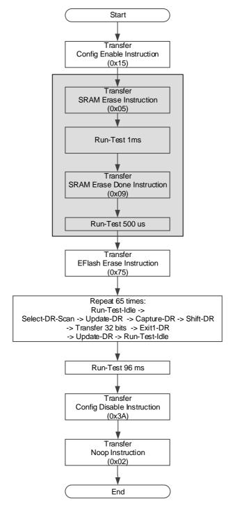
Figure 5-16 The Embedded Flash Erasing process of S Technology
