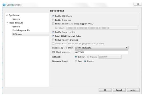
Gowin supports compressing bitstream data. The compression ratio is related to the user design. This manual only provides uncompressed configuration file sizes, as shown in Table 6-1.
