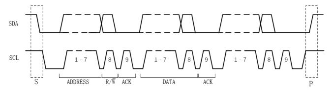
I<sup>2</sup>C is a serial transmission bus, which transmits data according to the protocol shown in the figure above. Under normal status, both SDA and SCL are at high level.
