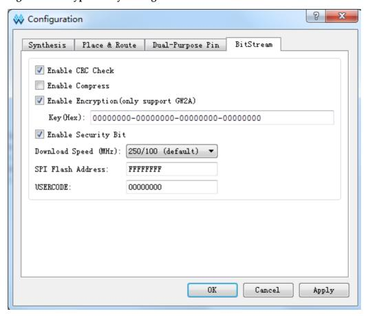
After setting the encryption key successfully, write the decrypted key to the FPGA key storage area for the device to analyze the encrypted bitstream data to complete the configuration.
