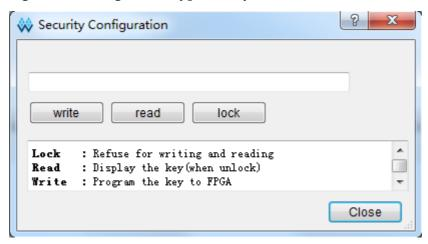
After the decryption key is written successfully, readback the written value via the "Read" button on the interface to verify.
