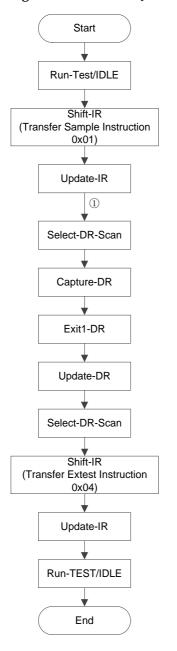
Figure 5-23 Transfer JTAG Instruction Sample & Extest Flow Chart
