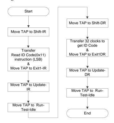
Figure 5-11 The Access Timing of Read ID Code Instruction-0x11
