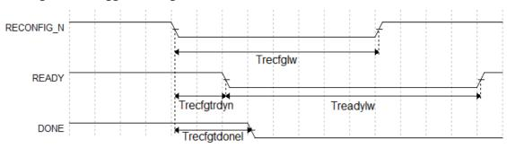
**Figure 5-3 Trigger Timing**
