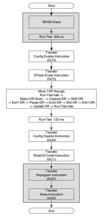
Figure 5-15 The Embedded Flash Erasing process of T Technology
