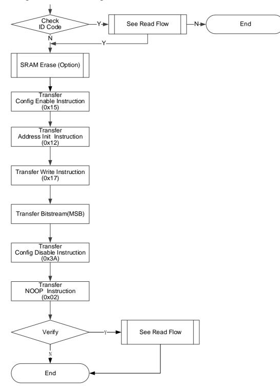
Figure 5-13 SRAM Configuration Flow
