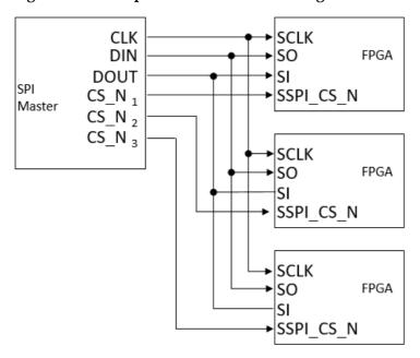
Figure 5-39 Multiple FPGA Connection Diagram 2
